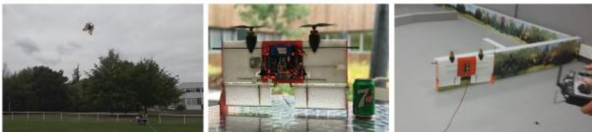
Figure 1: (i) MAVION during outdoors flight; (ii) MAVION next to a soda can for size comparison; (iii) MAVION during indoors flight.
