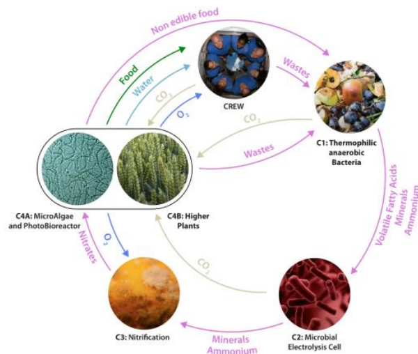
Figure 1: The concept of the MELiSSA loop with its five compartments and their interconnections. Picture from [11].
